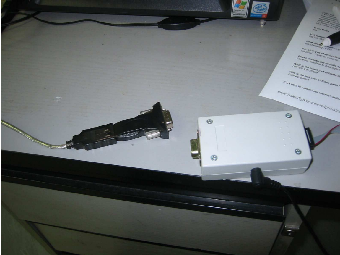
Figure 4.4.2 – Example of the serial connection removed from the SPC-2 box.
